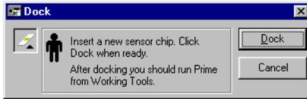
The docking operation takes a few seconds to complete. After docking, the **Working Tools** dialog box appears automatically with **Prime** highlighted as a reminder that you should run **Prime** after docking a new chip. For best results, you should also run **Working Tools:Normalize** after docking a new chip.
