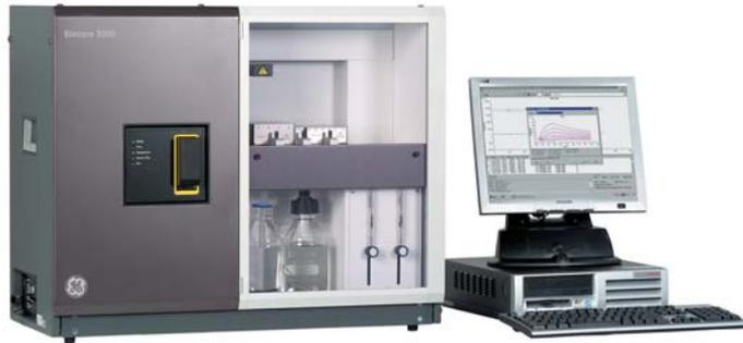
**Figure 2-1.** Biacore 3000 system processing unit and controlling computer.
