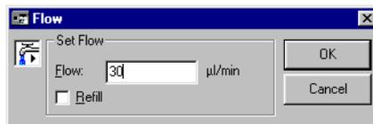
Enter the required flow rate in  $\mu\text{l}/\text{min}$  (permitted range 0-100  $\mu\text{l}/\text{min}$  in steps of 1  $\mu\text{l}$ ). To stop the flow, either choose **Command:Stop Flow** or set the flow to 0  $\mu\text{l}/\text{min}$  with **Command:Flow**.
