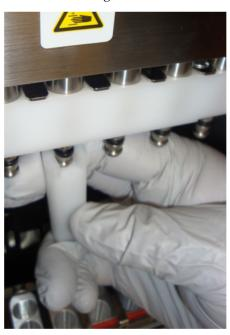
2. Using the D-ring installation tool, slip a new D-ring into the nozzle groove. Keep the flat inner surface of the D-ring in contact with the installation tool so that the D-ring does not roll. Ensure that the D-ring is placed properly on the nozzle to prevent leakage.
