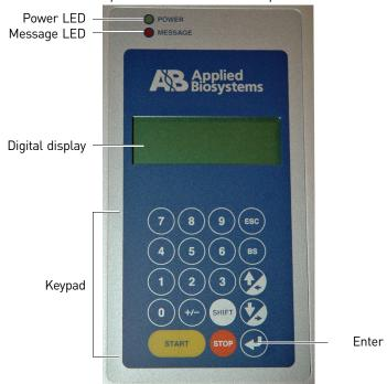
Figure 1 AutoMate Express™ Instrument – front panel
