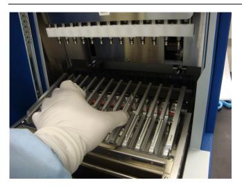
**5.** Insert the tip and tube rack into the instrument with row E in the front.
