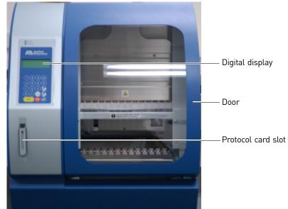
Figure 2 AutoMate Express™ Instrument – front view
