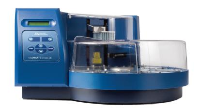
The MagMAX<sup>TM</sup> Express magnetic particle processors are ideal for automated magnetic-bead-based extraction of nucleic acids using the MagMAX Sample Preparation System. Two configurations are available: the MagMAX Express for low throughput processing, and the MagMAX Express-96 for high throughput environments
