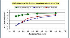
POROS MabCapture A media demonstrates higher dynamic binding capacity mostly independent of the residence time attained. Operational flow rate and column bed heights do not need to be optimized to allow for diffusion of the IgG to the rPA coated surface of the chromatography bead. Capture can be efficient and robust.
