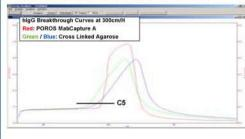
POROS MabCapture A media demonstrates higher breakthrough capacities for purified IgG as compared to a cross-linked agarose protein A affinity medias. Binding or capture of the IgG is steep and efficient, demonstrating the superb mass transfer capabilities of the media.
