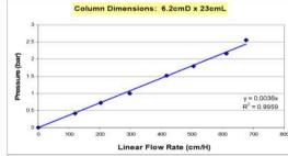
POROS MabCapture A exhibits a linear pressure response to increased flow rate. The media can be operated at high linear flow rates within common commercial system pressure limitations of 3 bar.
