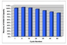
The capacity of the media is only slightly decreased after exposure to 0.1N NaOH, for 30 minutes per cycle at 500cm/H, for 50 sanitization cycles.
