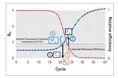
**Figure 5. The relative threshold (C**<sub>rt</sub>**) method.** The figure and steps below describe how the C<sub>rt</sub> is calculated. The amplification curve is in blue; the model of the reaction efficiency curve is in red; the y-axis on the left goes with the blue amplification curve, and the y-axis on the right goes with the red curve. C<sub>rt</sub> is determined in four steps:
