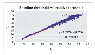
**Figure 2.**  $C_{rt}$  is strongly correlated to  $C_t$ . A total of 7,710 individual TaqMan<sup>®</sup> Assays with a wide range of  $C_q$  values (5–35) were run on the OpenArray<sup>®</sup> platform.  $C_{rt}$  and  $C_t$  values were generated for each throughhole, and strong correlation ( $R^2 = 0.9891$ ) was observed for the two methodologies.
