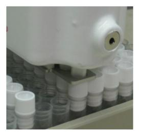
TIP: Line up the cap driver closest to the recharge socket with the tubes that are closest to you. The other drivers and tubes will then line up
