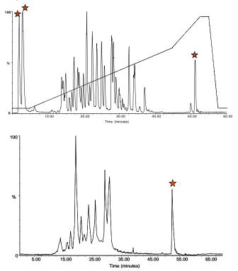
Figure 2. Total ion chromatogram (TIC) of tryptic digest of BSA in the presence of 1X Invitrosol<sup>TM</sup> solubilizer. Peaks indicated by stars correspond to components of the Invitrosol<sup>TM</sup> solubilizer. These peaks do not interfere with the peptide peaks.
