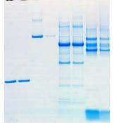
Figure 1. Separation of four protein samples on a 4-12% Bis-Tris NuPAGE<sup>®</sup> Gel before acetone precipitation, and after reconstituting the precipitated proteins in 1X Invitrosol<sup>™</sup> LC/MS Protein Solubilizer. Lane 1: myoglobin; lane 2: myoglobin/Invitrosol<sup>™</sup>; lane 3: BSA; lane 4: BSA/Invitrosol<sup>™</sup>; lane 5: P450-2D6; lane 6: P450-2D6/Invitrosol<sup>™</sup>; lane 7: AChR; lane 8: AchR/Invitrosol<sup>™</sup>.
