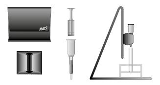
Attach MidiMACS™ Separator or QuadroMACS™ Separator to the MultiStand and place Whole Blood Column in the separator. Place a collection tube under the Whole Blood Column.
