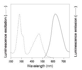
Figure 1. Luminescence excitation and emission spectra of SYPRO Ruby blot stain.
