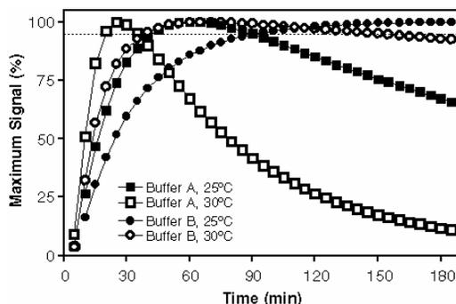
**Figure 1.** Gal-Screen assays were performed with purified  $\beta$ -galactosidase (500 pg) with either Buffer A or Buffer B. Repeated measurements were made in the Applied Biosystems TR717<sup>™</sup> microplate luminometer at either room temperature (25°C) or 30°C. Data is presented as percentage of maximum signal, and dotted line indicates 95% of maximum signal.
