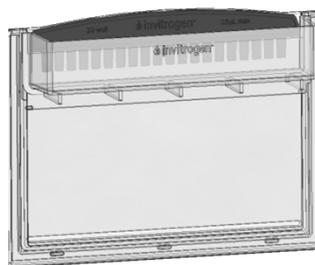
The attachment of the adapter on the gel cassette generates an **upper buffer chamber** that can hold ~75 mL running buffer and is required for use with the Criterion™ Cell.
