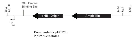
PLAC promoter: bases 75–104 (c) CAP protein binding site: bases 124–136 pMB1 origin of replication: bases 428–1,016 (c) Ampicillin (bla) resistance gene: bases 1,187–2,047 (c)
