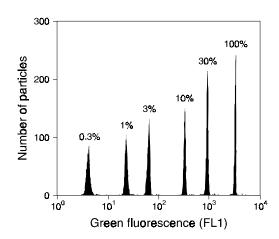
Figure 1. Fluorescence intensity histogram of the six fluorescent microsphere samples supplied in our InSpeck Green (505/515) Microscope Image Intensity Calibration Kit, 2.5µm. Fluorescence measurements were performed on a Becton Dickinson FACScan flow cytometer using excitation at 488 nm. The nominal relative fluorescence intensities are indicated; the actual measured values for this lot are 0.2%, 0.8%, 2.3%, 10.6%, 30.0%, and 100%, respectively.
