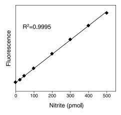
Figure 2. Linearity and sensitivity of the Measure-iT™ High-Sensitivity Nitrite Assay. Triplicate 10 µL samples of nitrite were assayed; fluorescence was measured at 365/450 nm and plotted versus picomoles of nitrite. Background fluorescence was not subtracted. The variation (CV) of replicate samples was <2%.
