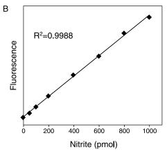
Figure 3. Extended Range for the Measure- $iT^{TM}$  High-Sensitivity Nitrite Assay. Triplicate 2  $\mu$ L (Panel A) or 20  $\mu$ L (Panel B) samples of nitrite were assayed using the Measure- $iT^{TM}$  High-Sensitivity Nitrite Assay. Fluorescence was measured at 365/450 nm and plotted versus picomoles of nitrite. Background fluorescence was not subtracted. The variation (CV) of replicate nitrite samples for both 2  $\mu$ L and 20  $\mu$ L volumes was <6%.
