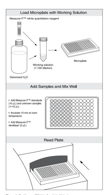
Figure 1. The Measure-iT™ High-Sensitivity Nitrite Assay.
