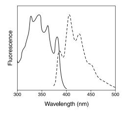
Figure 4. Normalized excitation and emission maxima for the Measure-iT™ nitrite quantitation reagent bound to nitrite.
