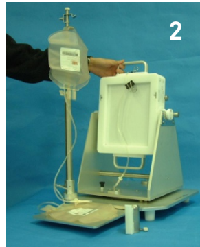
2. Tilt the Primary Magnet by 90°
