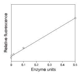
Figure 1. Detection of HIV reverse transcription using the Reverse Transcriptase Assay Kit, showing detection of 0.02 to 0.5 units of the enzyme. I unit = incorporation of 1 nmol of dTTP in 10 minutes at 37 °C, using poly(A) and oligo(dT) as the template and primer, respectively.
