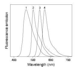
Figure 1. Normalized fluorescence emission spectra of the dyes contained in the FluoSpheres<sup>®</sup> fluorescent microspheres for tracer studies, after extraction into 2-ethoxyethyl acetate (Cellosolve<sup>®</sup> acetate). The four types of microspheres represented are: 1) blue-green, 2) yellowgreen, 3) orange and 4) red.
