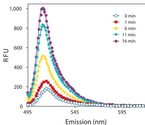
**Figure 2.** Plot of fluorescence emission intensities versus concentration of PLA<sub>1</sub> per well at 30 minutes, run at ambient temperature with liposomes. Fluorescence was measured exciting at 460 nm on a Spectra Max M5 (Molecular Devices). Background fluorescence determined for the no-PLA<sub>1</sub> enzyme control reaction has been subtracted.
