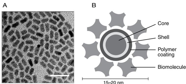
**Figure 1. A.** Transmission electron microscope image of core-shell Qdot® nanoparticles at 200,000x magnification. Scale bar = 20 nm. **B.** Schematic of the overall structure of a Qdot® streptavidin conjugate. The layers represent the distinct structural elements of the Qdot® nanocrystal conjugates, and are roughly to scale.
