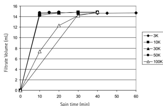
Spin conditions: 4,000 × g, room temperature, 15 mL starting volume. Protein markers used: Cytochrome c for 3K and 10K, BSA for 30K and 50K, and IgG for 100K, n=6.
