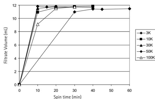
Spin conditions: 5,000 × g, room temperature, 12 mL starting volume. Protein markers used: Cytochrome c for 3K and 10K, BSA for 30K and 50K, and IgG for 100K, n=6.
