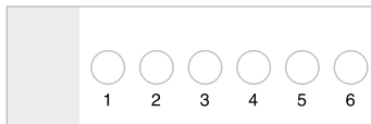
Figure 1. The TetraSpeck™ Fluorescent Microspheres Size Kit includes a sample of each size of TetraSpeck™ microspheres mounted on one slide. Position 1 contains 4.0 μm microspheres; position 2 contains 1.0 μm microspheres; position 3 contains 0.5 μm microspheres; position 4 contains 0.2 μm microspheres; position 5 contains 0.1 μm microspheres; and position 6 contains a mixture of all of the sizes.
