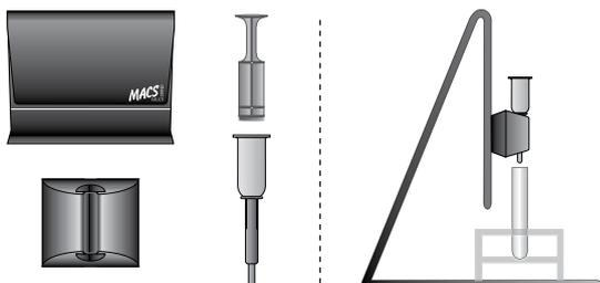
Attach MidiMACS™ Separator or QuadroMACS™ Separator to the MultiStand and place LS Column in the separator. Place a collection tube under the LS Column.
