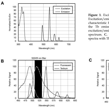
Figure 1. Excitation/emission spectra for Tb chelates. A. Excitation/emission spectra for Tb chelates. Note the characteristic four sharp peaks with baseline separation in the Tb emission spectrum. B. Overlap of fluorescein excitation/emission spectra with Tb chelate emission spectrum. C. Overlap of rhodamine excitation/emission spectra with Tb chelate emission spectra with Tb chelate emission spectra.
