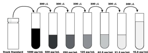
Serial dilutions within the plate may also be performed by pipetting 100 µL of Assay Diluent into each standard well except the highest (1000 pg/mL), then adding 100 µL of the 1000 pg/mL standard to both that well and the 500 pg/mL well, mixing the well contents by rinsing the pipette tip, and adding 100 µL of the 500 pg/mL standard to the 250 pg/mL well. Continue these dilutions to the 15.6 pg/mL standard well, out of which the extra 100 µL should be discarded.
