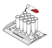
**Note:** If all the samples have not passed through the filters in the specified time, run the vacuum for additional time until all samples are completely evacuated.
