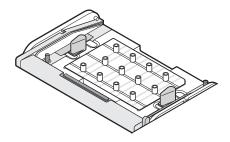
b. Label the filter vials, then insert a filter vial into each port on the adapter plate.
