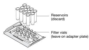
b. Clean the filter vials, including the rims, by pipeting RNA Purification Wash Solution I into each filter vial, then apply vacuum until all wash solution is completely evacuated.
