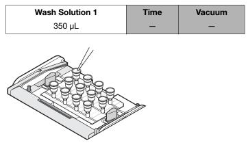
d. Attach a 15-mL reservoir to the top of each of the filter vials.
