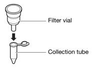
b. Pipet Nucleic Acid Purification Elution Solution into each filter vial and allow the elution solution to completely soak the filters.
