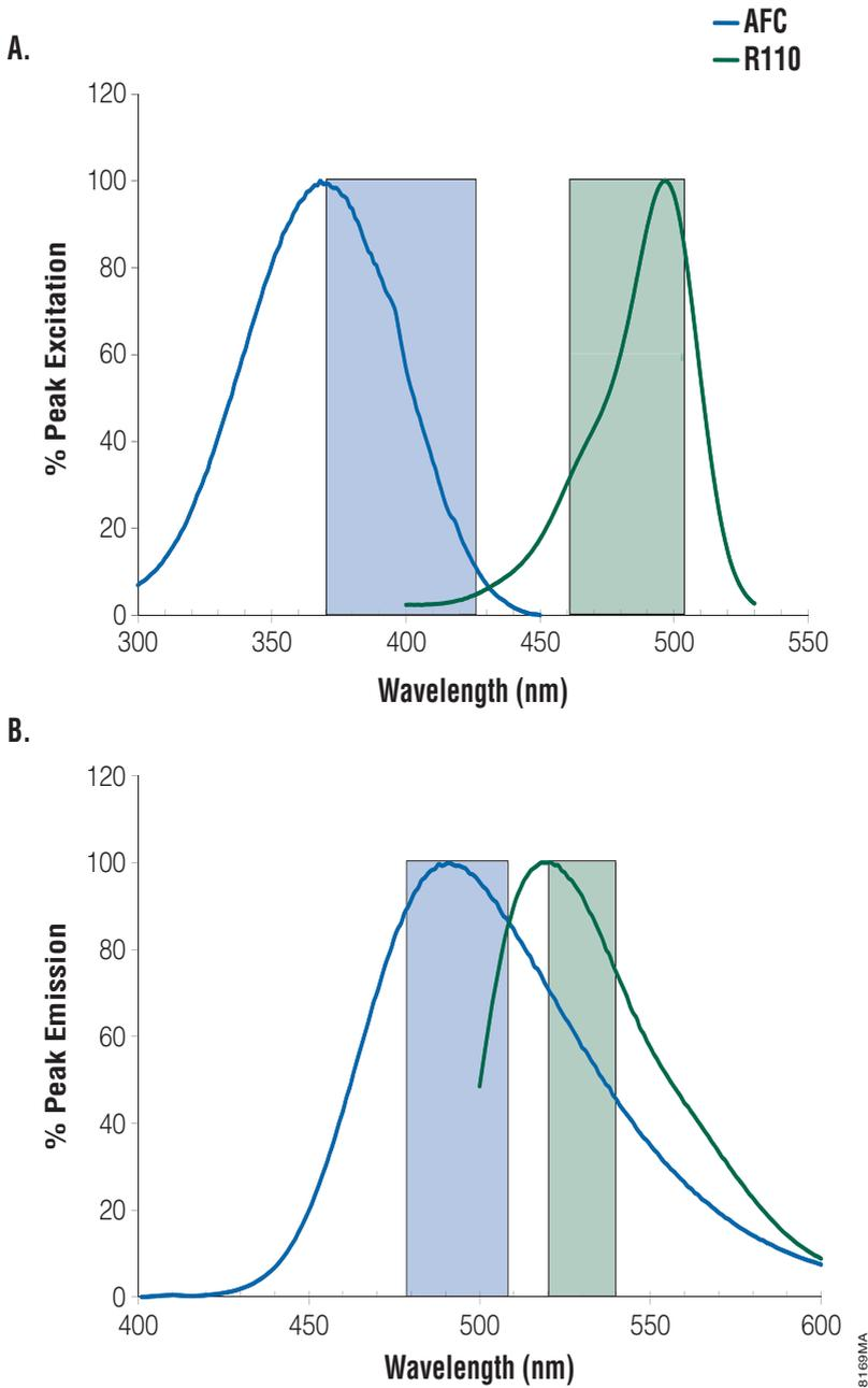
**Figure 8. Peak excitation and emission wavelengths for the GF-AFC and bis-AAF-R110 Substrates.** Boxes indicate the optimal filter sets ranges required for separating and measuring the fluorescence signals.
