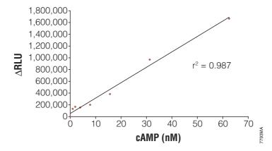
**Figure 4. Titration of purified cAMP.** Reactions were assembled with the indicated concentrations of purified cAMP in a white standard 384-well plate. The cAMP-Glo™ Assay was performed as described in Section 5.A. Data were collected using a plate-reading luminometer (FLUOstar OPTIMA, BMG Labtech). Each point represents the average of four data points. Data analysis was performed with Excel using linear regression.
