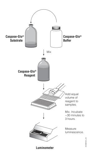
Figure 3. Schematic diagram of the Caspase-Glo® 3/7 Assay protocol.
