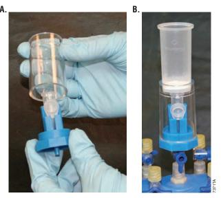
**Figure 3. Elution by vacuum. Panel A.** A 1.5ml microcentrifuge tube is placed in the base of the Eluator<sup>TM</sup> Vacuum Elution Device (Cat.# A1071) with the tube cap secured in the open position. **Panel B.** The Eluator<sup>TM</sup> Vacuum Elution Device assembly, including the binding column, ready for use on a vacuum manifold.
