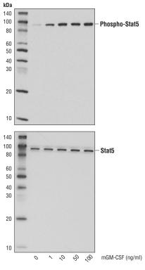
Western blot analysis of extracts from MC/9 cells untreated or treated with mGM-CSF for 10 minutes, using Phospho-Stat5 (Tyr694) (C11C5) Rabbit mAb #9359 (upper) and Stat5 (3H7) Rabbit mAb #9358 (lower).
