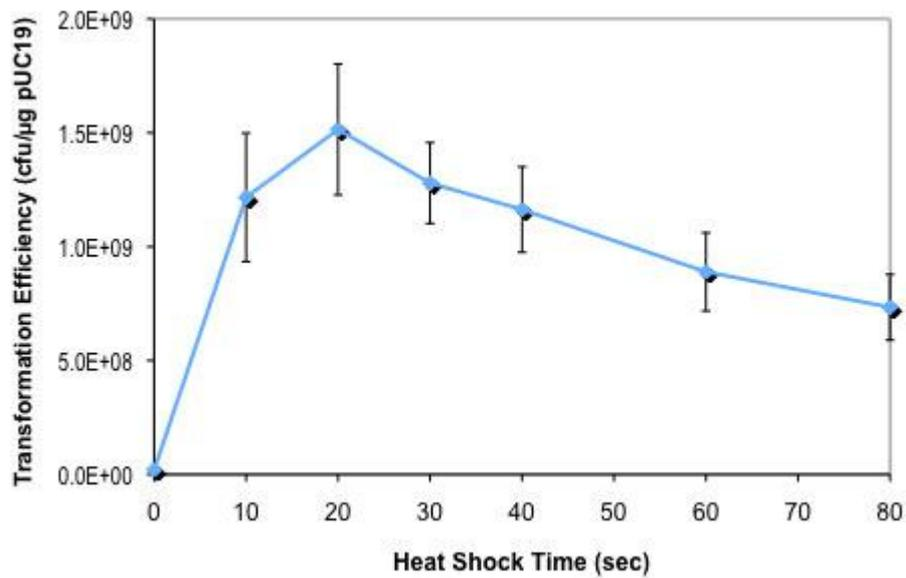
**Effect of heat shock time on NEB Express competent *E. coli* transformation efficiency:** 50 µl of competent cells were transformed with 100 pg of pUC19 control DNA following the provided High Efficiency Transformation Protocol except heat shock time varied from 0 to 80 seconds.
