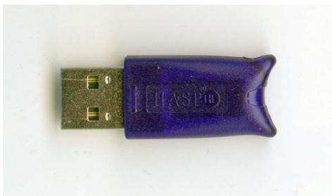
If the software activation dongle is not detected, the following warning will appear: "Sentinel HASP key not found (H007)".
