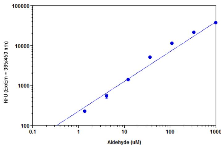
**Figure 1.** Aldehyde dose response was measured in a solid black 96-well plate with Amplite™ Fluorimetric Aldehyde Quantitation Kit using a Gemini fluorescence microplate reader (Molecular Devices). As low as 3  $\mu\text{M}$  of aldehyde can be detected with 15 minutes incubation ( $n=3$ ). *Note: The fluorescence background increases with time, thus it is important to subtract the fluorescence intensity value of the blank wells for each data point.*
