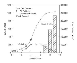
**Figure 3.** CELLIGEN<sup>TM</sup> was seeded with Sf9 cells at 2 x 10E5 cells/mL and infected on day 4 post-planting with rAcNPV (construct VL-941) at MOI of 0.50 when the culture reached 2 x 10E6 cells/mL. Bioreactor was sampled daily post-infection for  $\beta$ -GAL expression.
