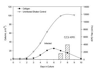
**Figure 4**. CELLIGEN<sup>TM</sup> was seeded with Sf9 cells at 2 x 10E5 cells/mL and infected on day 5 post-planting with rAcNPV at a MOI of 0.50 when the cell density reached  $2.5 \times 10E6$  cells/mL. The culture was sampled daily post infection for rEPO.
