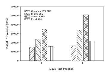
**Figure 1.** 250 mL shake flask cultures were seeded at 3 x 10E5 cells/mL (100 mL volume). The cultures were infected on day 4 post-planting with rAcNPV at a MOI of 0.50 when the cell densities reached 3 x 10E6 cells per mL.  $\beta$ -Galactosidase was assayed on days 4 and 6 post-infection.
