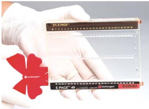
2. Gently pull apart the cassette halves with your hands until the cassette halves are completely separated and the gel is exposed.
