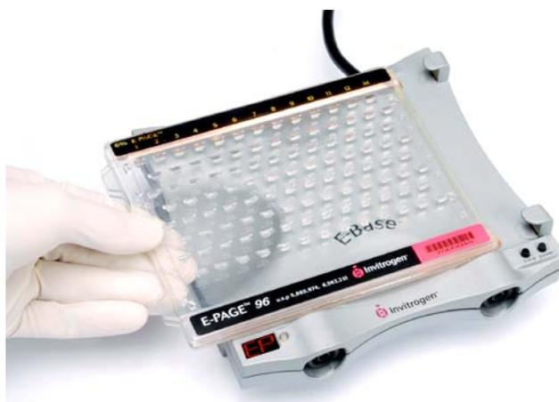
When the gel is properly inserted into the base, a fan in the base begins running, and a red light illuminates at the lower left corner of the base. The digital display shows the appropriate time for a selected program or the last time setting (Ready Mode).
