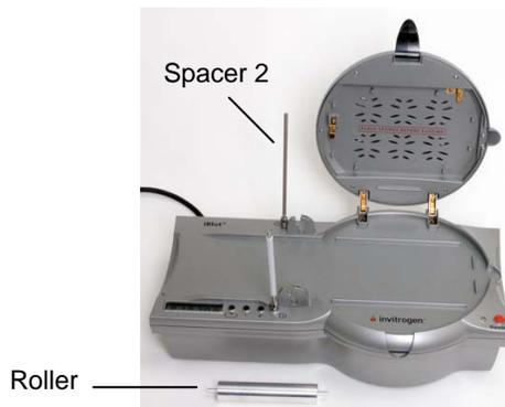
2. Remove the package labeled iBlot<sup>®</sup> Anode Stack, Bottom from the iBlot<sup>®</sup> Gel Transfer Stacks Box. Remove the laminated sealing of the iBlot<sup>®</sup> Anode Stack, Bottom and **keep the stack in the transparent plastic tray**.
