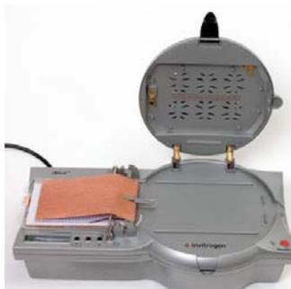
10. Insert the De-bubbling Roller into the two grooves and lower the roller to its lowest location while holding the pull tab. The resulting assembly consists of the gel, and cathode and anode stacks placed between two Metal Spacers 1 and 2 with the De-bubbling Roller on top of the assembly as shown below.
