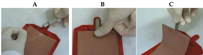
9. Place the iBlot<sup>®</sup> Cathode Stack, Top **without the tray** on top of Metal Spacer 2 with the copper electrode side facing up (and agarose side facing down). Ensure that all layers are aligned to the right to perform efficient de-bubbling.
