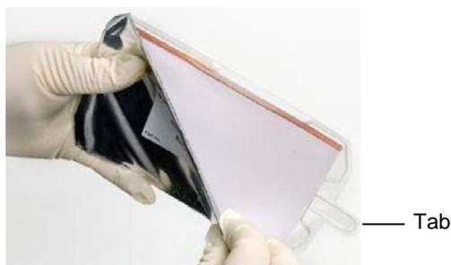
3. Place the iBlot<sup>®</sup> Anode Stack, Bottom stack **with the tray** to the left of the blotting surface area such that the tab on the tray is on the right side of the De-bubbling Roller, as shown below. Slide the bottom stack to the left until the stack is blocked by the Gel Barriers present on the left side of the device.
