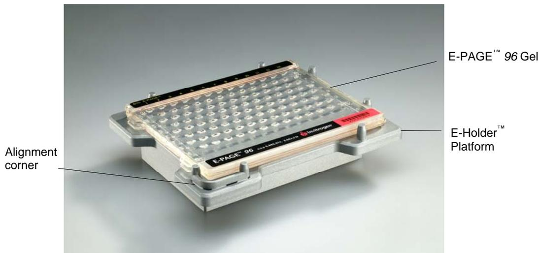
4. **Optional:** Set up your automated liquid handling system to load samples into the E-PAGE™ 48 or 96 Gel placed on an E-Holder™ Platform. Program your automated liquid handling system to load the samples approximately 5 minutes before the previous electrophoresis run is complete. This ensures that the loaded gel from the E-Holder™ Platform is placed onto an E-Base™ Device within the recommended time of 15 minutes.
