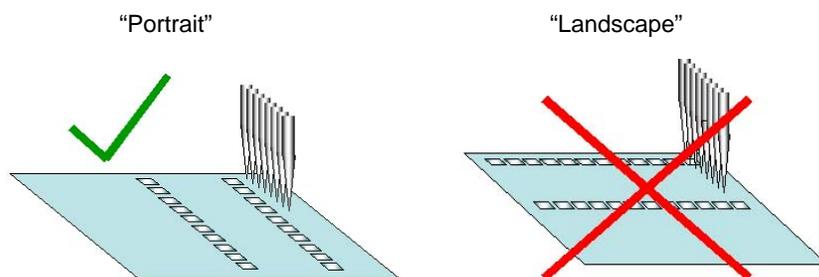
This orientation is available for some automation systems with the use of a 90° adapter. If your system does not have an adapter that allows the “Portrait” configuration, please contact Technical Support (page 72) to obtain a 90° adapter.
