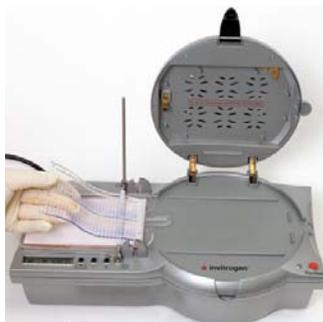
6. Clean the Metal Spacer 2 with a damp cloth or tissue and place the spacer over the gel as shown below.
