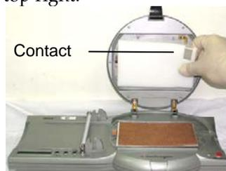
The sponge absorbs any excess liquid generated during blotting and exerts an even pressure on the stack surface.
