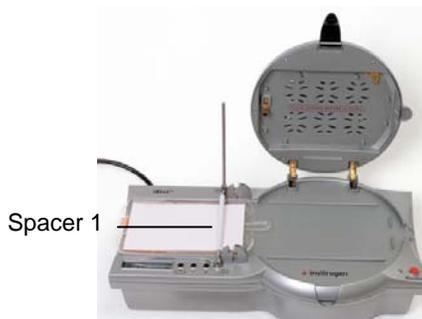
5. Place the prerun gel containing your protein samples on Metal Spacer 1 such that the gel is aligned to the lower right corner of the bottom stack with the wells of the E-PAGE<sup>™</sup> gel facing up.
