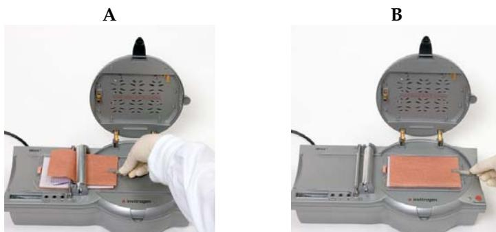
12. Place the iBlot<sup>®</sup> Disposable Sponge on the inner side of the lid (between the small protrusions on the lid that hold the sponge in its place) such that the metal contact is to the top right.
